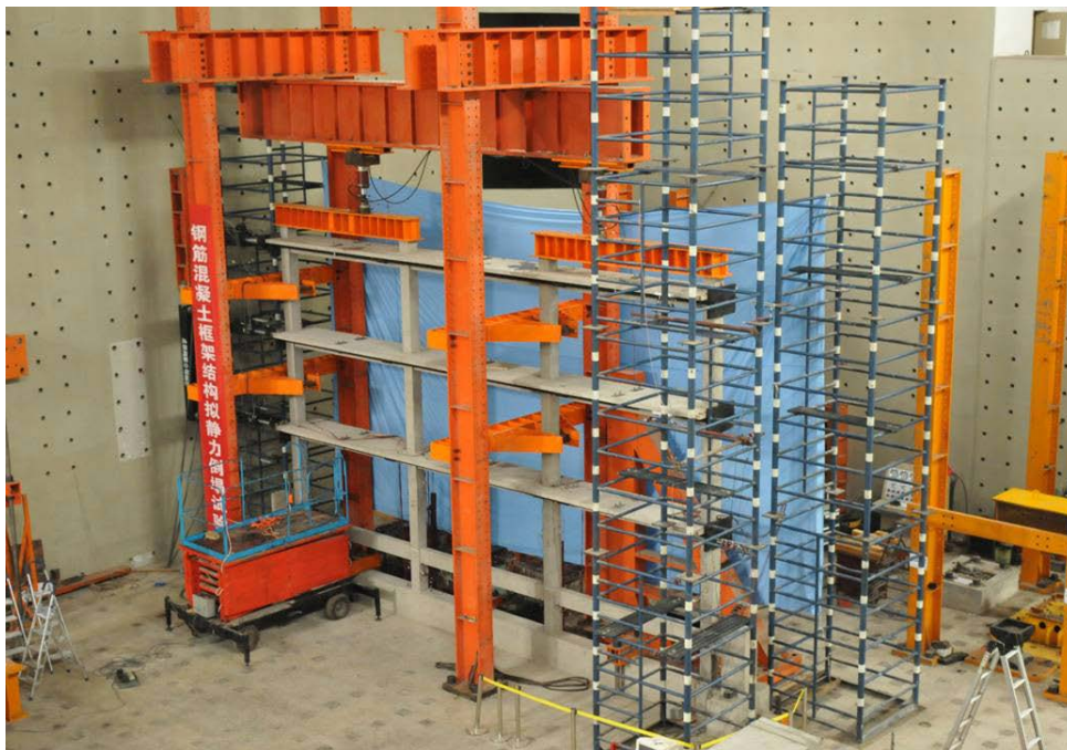
Figure 4.111. Half-scale, three-storey reinforced concrete frame tested under pseudo-static cyclic loadings
