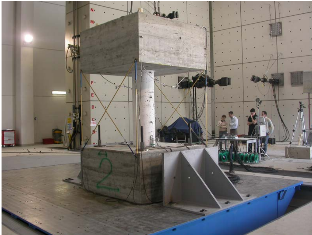
Figure 4.85. Bridge pier tested at the EUCENTRE
