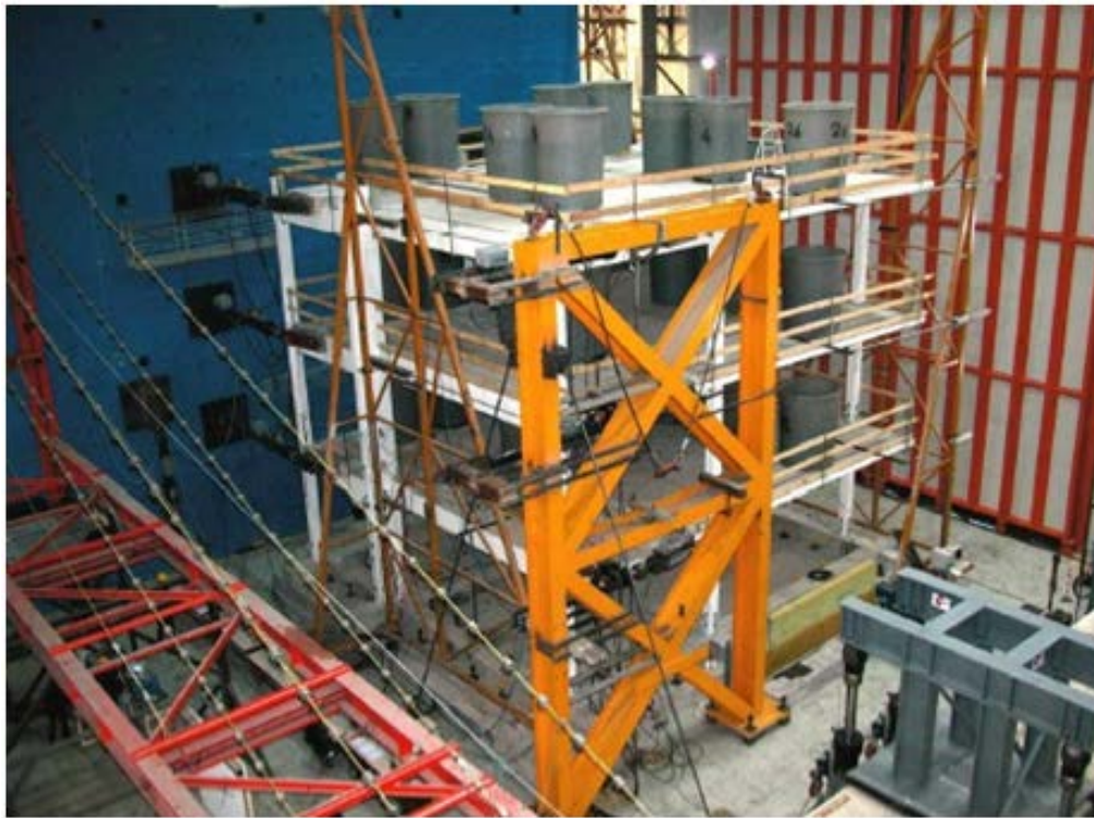
Figure 4.16. Full-scale, three-storey prototype building [Fardis & Negro, 2006]
