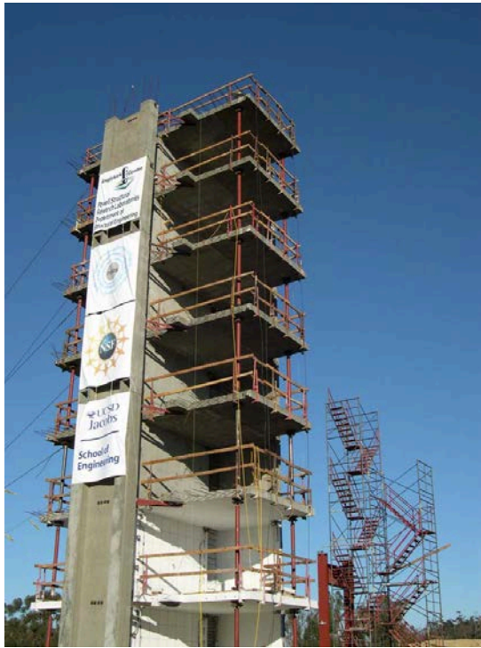
Figure 4.9. Seven-storey, full-scale RC shear wall building tested at the NEES Large High-Performance Outdoor Shake Table at UCSD's Englekirk Structural Engineering Center [Martinelli P. and Filippou F.C., 2009]
