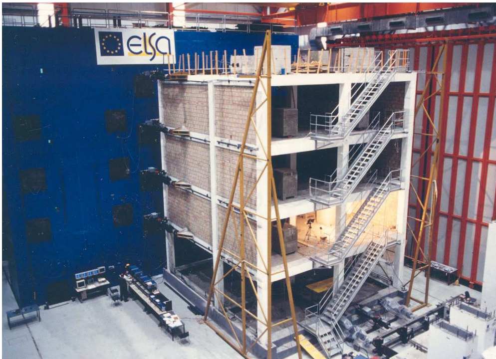
Figure 4.46. Four-storey 3D infilled frame tested by Negro et al. (1996)
