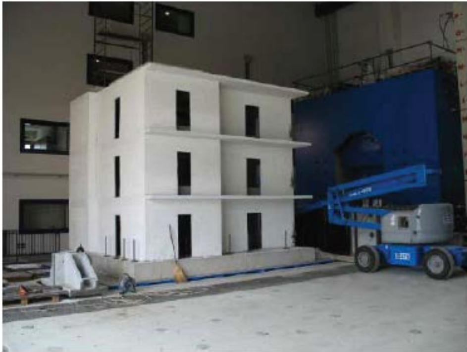
Figure 4.57. Half scale, three-storey infilled RC building
