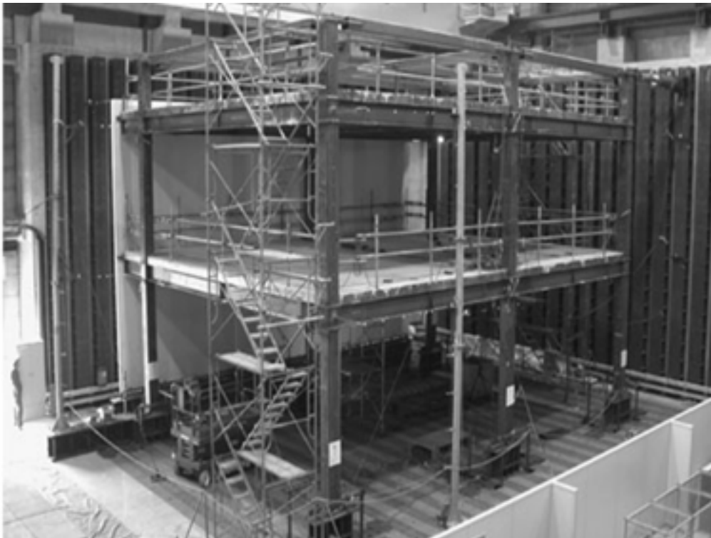
Figure 4.23. Three-storey, three-dimensional steel moment frame [Nakashima et al., 2006]
